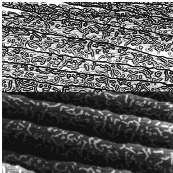
Figure 3. Composite STM image (raw data and enhanced edge contrast) of methyl pyruvate on Pt{111} at 298 K in the absence of hydrogen showing the formation of polymeric chains [constant current mode, 1000 \text{ \AA} \times 1000 \text{ \AA} , U_{\text{gap}} = -1 \text{ V} , I_T = 10 \text{ nA} ].
